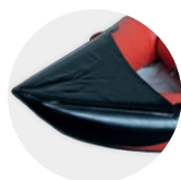
(b) REINFORCED FABRIC POINT
